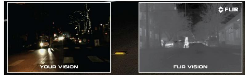
The above images show a comparison of typical night time driving compared to using the Helios thermal imager. The image on the left is from an ordinary digital camera and shows the amount of visible light as illuminated by oncoming headlights. The image on the right is a thermal image created by the Helios thermal imaging camera. Note the Helios camera is sensitive to warm objects, such as the people, and provides visibility over a much greater distance.
