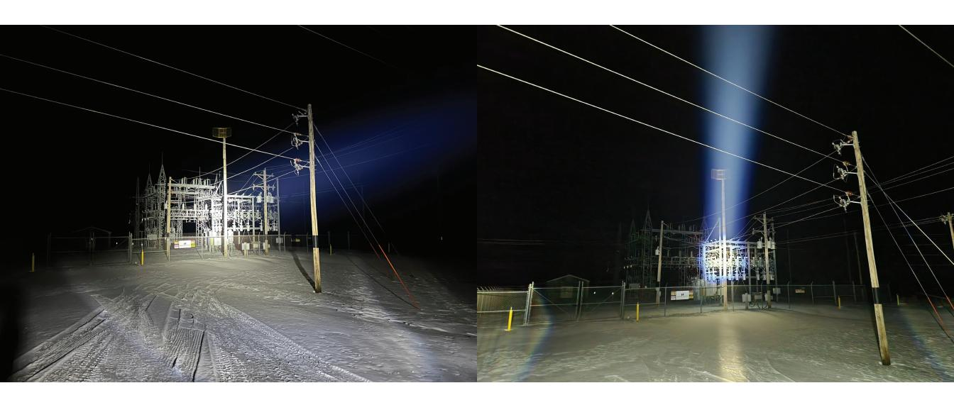
Image Left - LED Hybrid Image Right - LED Spot @300 ft from Bins
