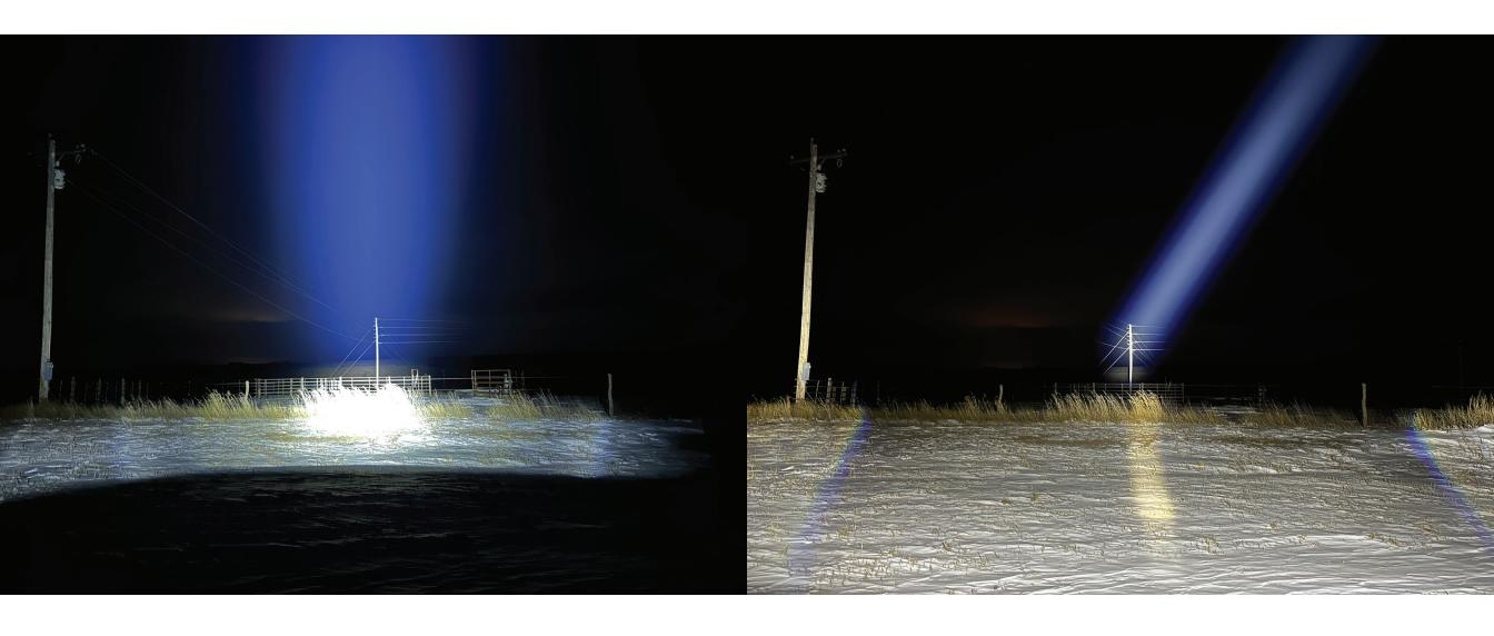
Image Left - LED Hybrid Image Right - LED Spot Poles on right @ 260 ft apart
