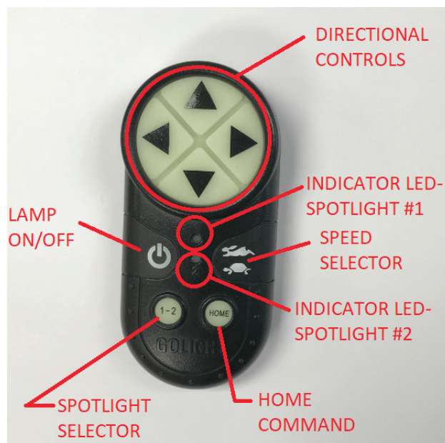
Figure 5 – Stryker® ST Wireless Handheld Remote Features
